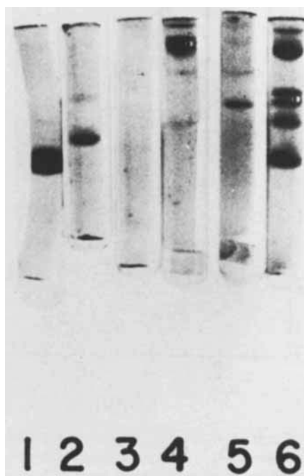
Fig. 3. SDS-acrylamide gel electrophoresis of a urate oxidase preparation and marker proteins: Gel 1, cytochrome c; Gel 2, chymotrypsinogen A; Gel 3, blank; Gel 4, bovine serum albumin; Gel 5, urate oxidase; Gel 6, mixture of all samples. Conditions are as described in the text.
